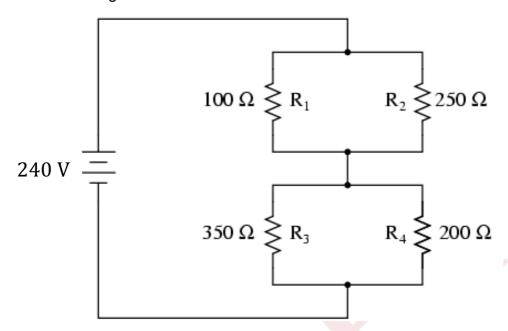
(a) Calculate the total resistance of the circuit.
