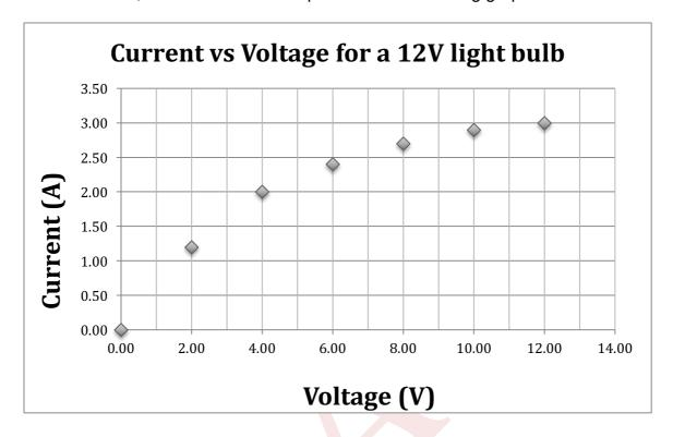
(a) Calculate the resistance of the light bulb at the intended operating voltage of 12.0 V.
