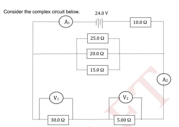
(a) Calculate the total resistance of the circuit.
